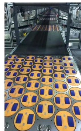
DWS扫码称重与旋转轮分拣线 The DWS sorting line, include barcode scanning, weighing, rotary wheel sorter.
