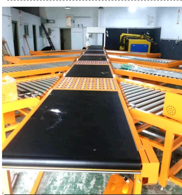
The DWS line introduce Scanning, weighing, and rotary wheel sorting line
