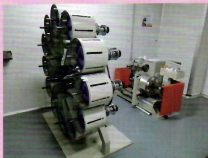
废纤收卷机 Waste fiber winding machine
