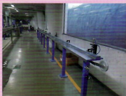
余长测试台 E.F.L measure device
