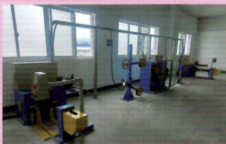
束管复绕机 Loose tube rewinding machine
