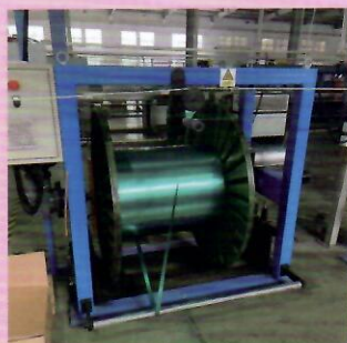
大盘钢铝带放带 Big reel steel and aluminum tape pay-off
