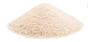
Silica sand consists mainly of silica (silicon dioxide), which has delicate and hard grains. In water purification, silica sand is used as a filtration medium to remove impurities, solid particles, and contaminants in water.
