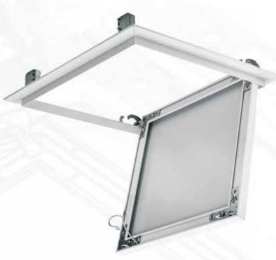
PROSTAR Aluminum access panels are applied from the top to the places where they will be installed. Due to the teethed structure of the inner frame inside the cover, there is no need to remove the plaster after application. It is painted and the assembly is completed without any delay. Prostar plasterboard access panels are suitable for 12.5 mm thick plasterboards
