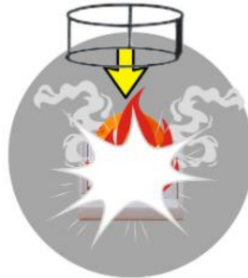
Step - 3 The ball activates within 3-5 seconds and explode.
