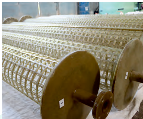
CANDLE FILTERS WET CHLORINE, P2O5, ETC APPLICATIONS 80% OPEN AREA WITH 99.9% FILTRATION EFFICIENCY, LOW PRESSURE DROP, MAXIMUM SURFACE CONTACT
