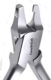
CW-2932 Vertical Punch Plier This versatile plier emphasizes on over-correction of rotations by creating an indentation at the mesial and/or lingual of a specific tooth. Can also be used to create a rotational couple using vertical indents on facial and lingual surfaces on opposite sides of a tooth.
