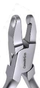
CW-2931 Hole Punch Plier Creates half-moon cutouts in clear aligners to allow space for bonded buttons used for elastics
