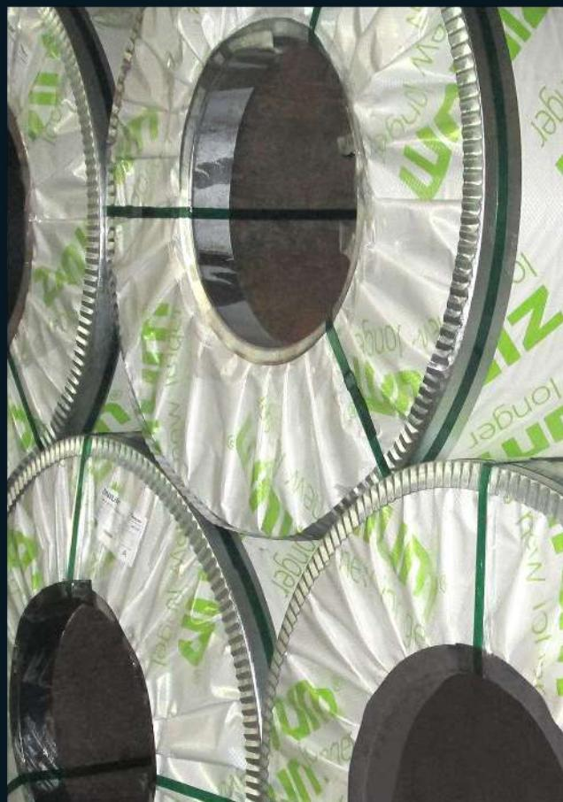
To protect product during distribution and storage, as well as to extend the life of coils against corrosion, careful and well packaging is required. The way PT. SUNRISE STEEL package their products is illustrated in the picture.
