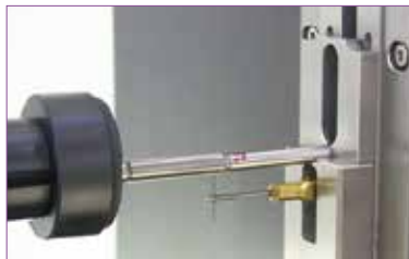
Coaxiality of lead screw
