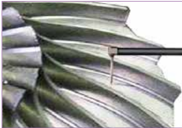
Ra of engine blade
