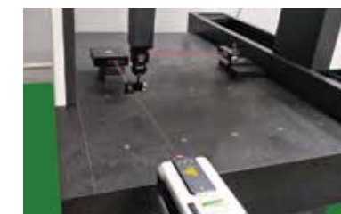
Perpendicularity meas. of CMM
