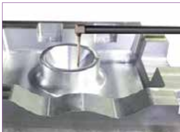
Ra & Profile of mold
