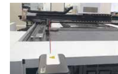
Straightness meas. of equipment
