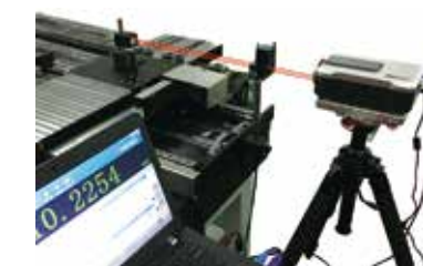
Linear meas. of stage module
