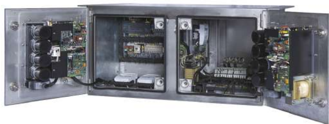
ENERGY SUPPLY AND COOLING CONTROL SYSTEM
