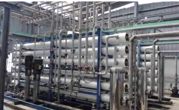
Project Name : A landfill project in Zhejiang *Recovery Rate > 96% ( up to 98% ) *Treated water color 0 *Treated water met RO feed requirement *NF system operation pressure 0.48-0.80Mpa
