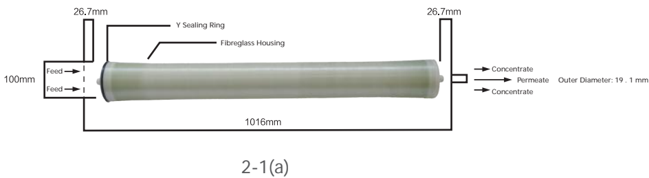
E-MEM® Industrial 8040 Membrane Element Dimension Diagram
