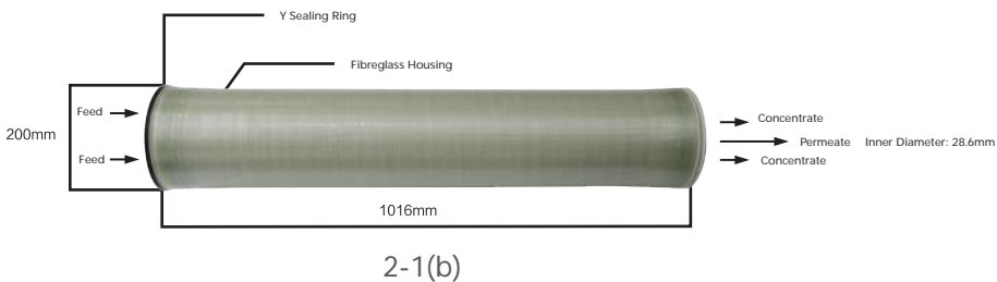
E-MEM® Industrial 8040 Membrane Element Dimension Diagram
