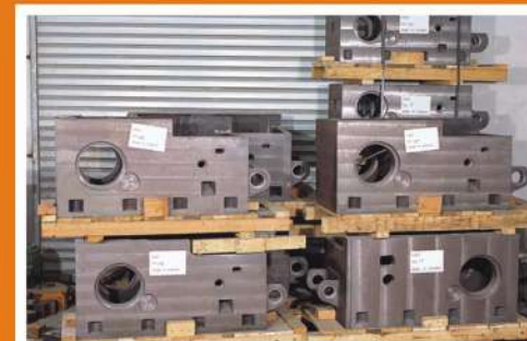
冷鍛成型機之本臺鑄件 (臺灣進口) Taiwan Imported Main Frame of Cold Former
