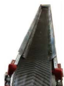
皮带机 Belt Conveyor
