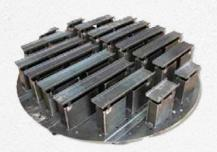
Chimney Collector trays are used to gather liquid from packed beds during tray transition. They are needed in various situations, like drawing off liquid either partially or completely. There are different types of these trays to fit the amounts of vapor and liquid.
