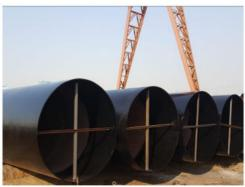
Product Dimension: WELD: Φ219-3000mm, WT:6mm-200mm, Length: 3.0m-200m Standard: API SPEC 5L PSL1&PSL2, ISO 3183, A53, ASTM A500, ASTM A252, ASTM A671, ASTM A672, ASTM A691, EN10210, EN10217, EN10219 etc
