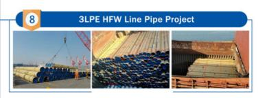
HFW API 5L B 660.4\*9.53\*12m Coat Type:Zinc Rich Epoxy Primer+Epoxy poly amide mid-Coat+Polyurethane Top-coat,962tons
