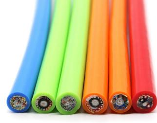
Derul sewer inspection camera cables are used to operate sewer cameras, sewer robots and sewer renovation systems. Sewer inspection camera cables typically comprise a coaxial cable as a camera cable for transferring video signals and several conductors to control and illuminate the camera system, which is usually self-propelled.
