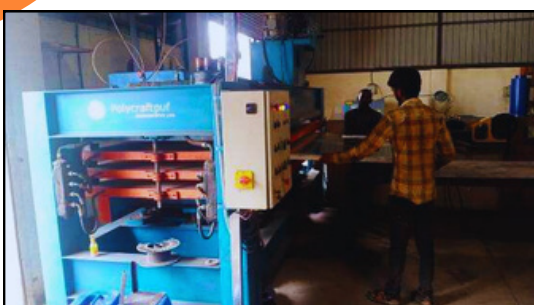
Hot Press of Doors for Rigidity
