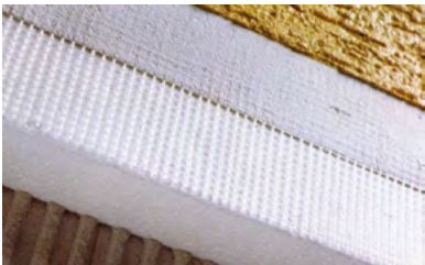
装饰砂浆饰面外墙外保温样板 Exterior wall external insulating sample plate with decoration mortar
