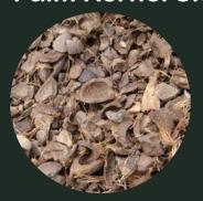
Palm kernel shell is a by-product in the production of palm oil and is commonly used in the natural biomass energy industry. Due to its high calorific value, averaging 4000 Kcal/kg, and low ash content, it is considered an attractive source of fuel in the production of energy from renewable sources.
