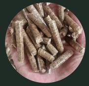
Solid fuel made from compressed organic material. Pellets can be made from any one of five general categories of biomass: industrial waste and coproducts, food waste, agricultural residues, energy crops, and untreated lumber. Wood pellets are generally made from compacted sawdust and related wood industrial wastes.
