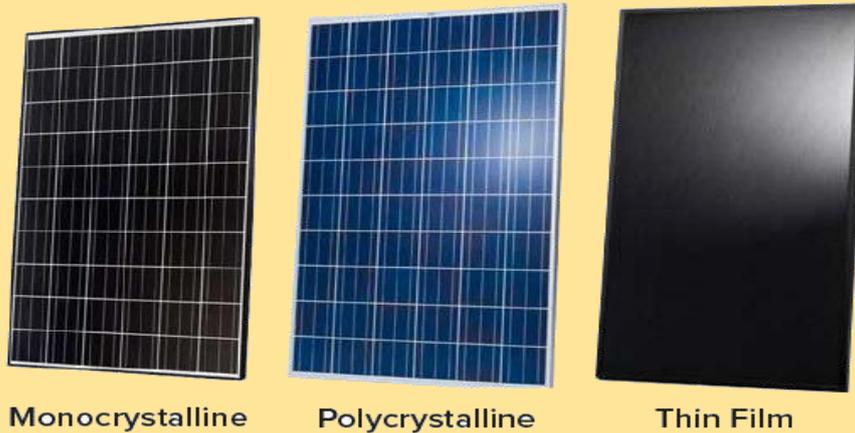
Vary in the composition of the silicon itself. Monocrystalline solar cells are cut from a single, pure crystal of silicon. Alternatively, polycrystalline solar cells are composed of fragments of silicon crystals that are melted together in a mold before being cut into wafers.
