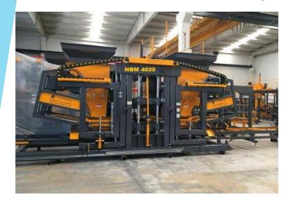
The production capacity is 2600-3000 pieces per hour and it is able to produce paving stone and briquettes in capacities ranging from 1500-2000 units. manual, semiautomatic and full automatic preferred fixed machines.
