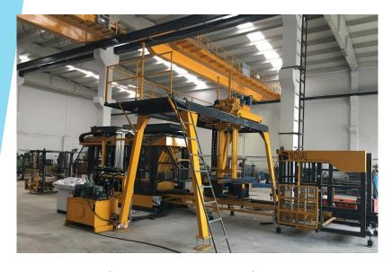
Production capacity of 3500-3800 pieces per hour, and it is able to produce paving stone and briquette production capacity between 2000-2500 unites. semi-automatic and fully automatic preferred fixed machines.
