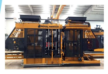
Production capacity is between 5000-5500 pieces per hour and it is able to produce briquettes in capacities ranging from 3500-4000 units. manual, semi-automatic and full automatic preferred fixed machines.
