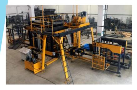
Production capacity between 4000-4600 pieces per hour and the production of paving stones and briquettes production in capacities ranging from 2500-3000 units. semi-automatic and fully automatic preferred fixed machines.
