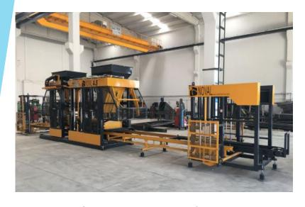
Production capacity is between 1500-1900 pieces per hour and it is able to produce paving stone and briquettes in capacities ranging from 800-1000 pieces. manual, semi-automatic and fully automatic preferred fixed machines..
