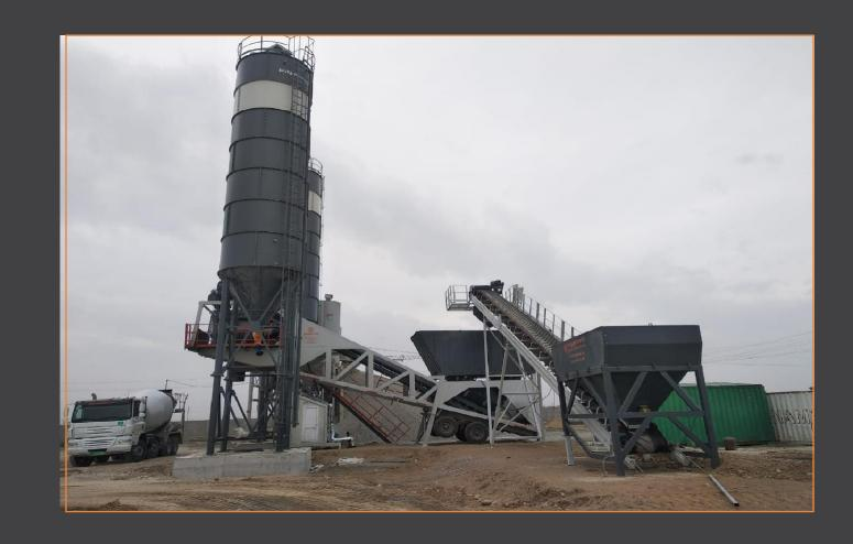
Aggregate hopper can be filled through a concrete/steel aggregate loading ramp or more effectively through Aggregate Pre-Feeding System. There are two types of Aggregate Pre-Feeding System.
